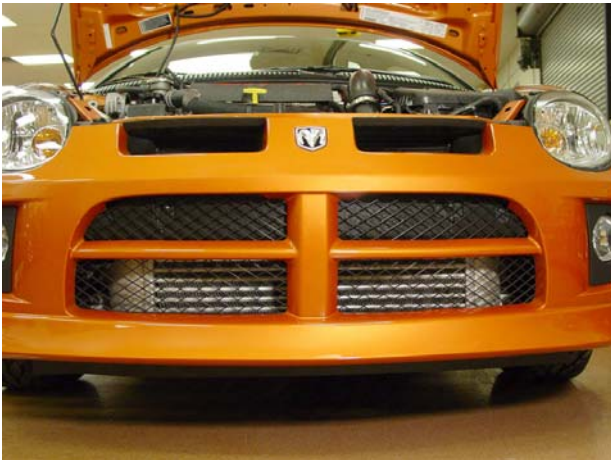
Figure 14 – The stock SRT-4 intercooler is only visible in the lower half of the grille.
