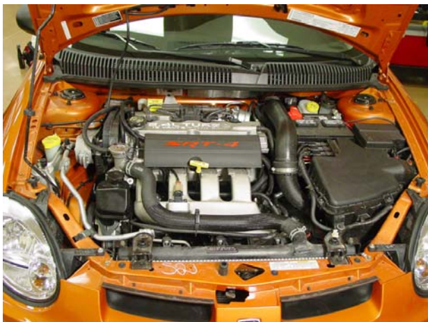
Figure 10 – Note the air intake path in the stock SRT-4 engine compartment.
